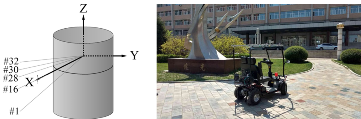
Fig. 1. System configuration; here, the distribution of LIDAR harness (a) and the installation of LIDAR (b).
