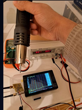
a) hot air significantly decreases the output power
