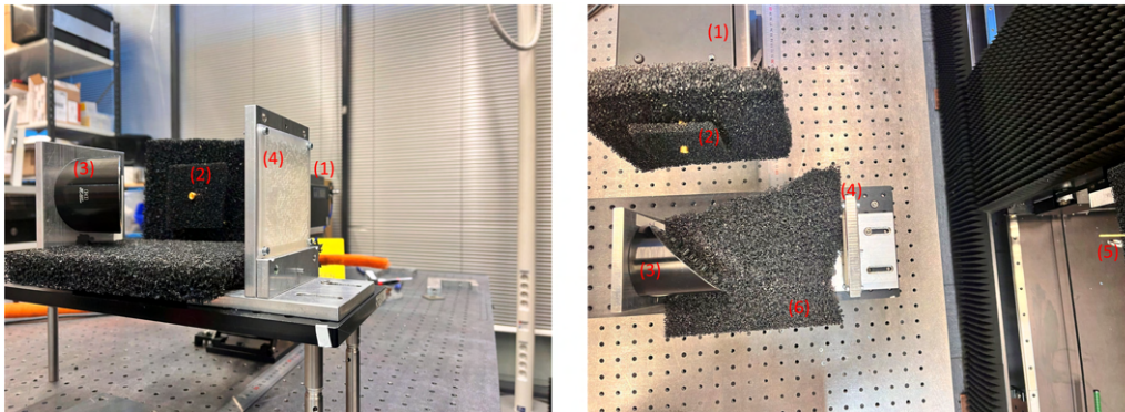
Figure 5.1: Photography of the imaging setup at 220-330 GHz. 1) WR3.4-VNAX transceiver; 2) Pickett-Potter horn antenna; 3) OAP mirror; 4) holograms; 5) OEWG probe antenna connected with to WR3.4-VNAX receiver. 6) RAM
